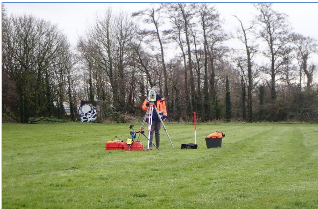
Plate 1: Base station set-up with Total Station EDM.
